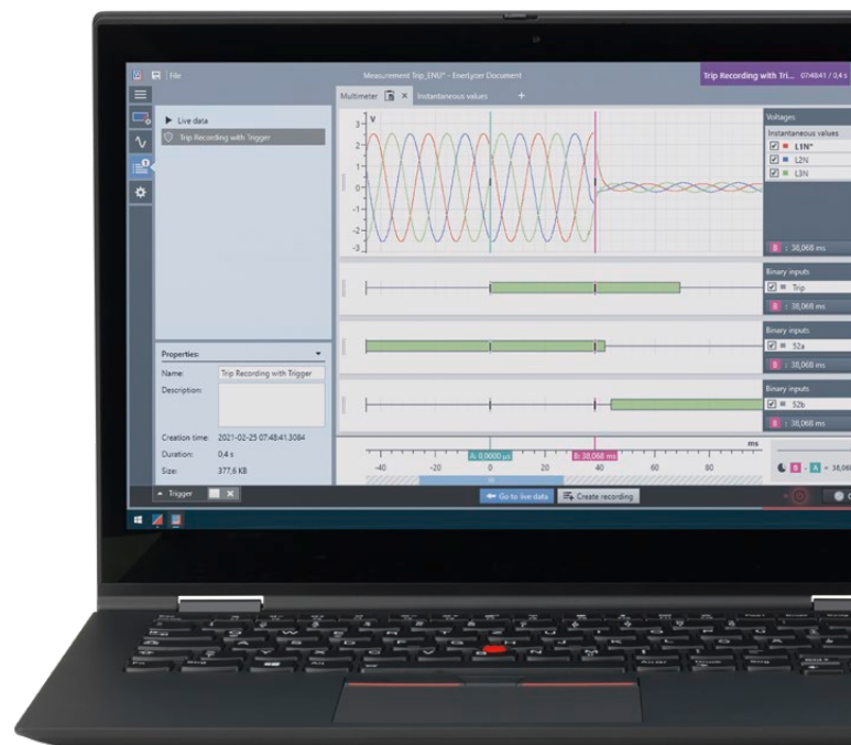
Open/close timing measurement of a circuit breaker with EnerLyzer
